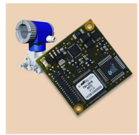
incurred. The board is designed according to the specifications of the Fieldbus Foundation and the PROFIBUS Trade Organization and is ready to pass all necessary conformance testing.
